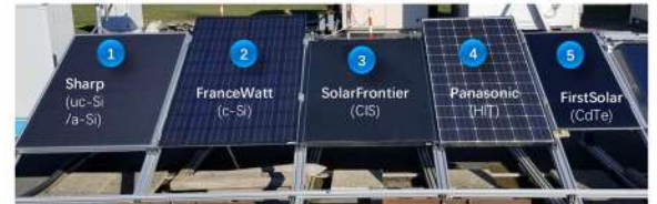
Figure 1: PV modules in SIRTA with 5 different technologies under operation since 2014
