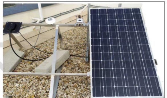
Figure 2: Outdoor DUSST sensor side-by-side with an automatic soiling station as well as a pyranometer installed at the University of Jaén, Spain.
