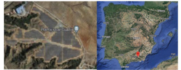
Figure 2: Left: Aerial photograph of the PV plant. It has a nominal capacity of 4.4 MWp. Right: Location of the plant within Spain. The plant is located in the southeast of Spain. The average annual horizontal solar irradiance is higher than 1800 kWh/m 2 .
