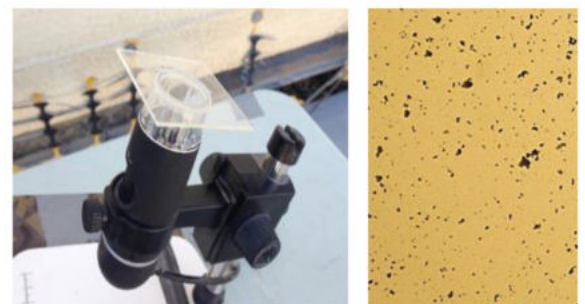
Figure 3: (left) a front soiling microscope (right) photo taken with the microscope
