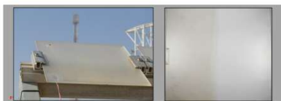
Figure 2: Testing of functional surfaces on glass at the Negev Desert; Same sample after 2 years, half side cleaned for characterization
