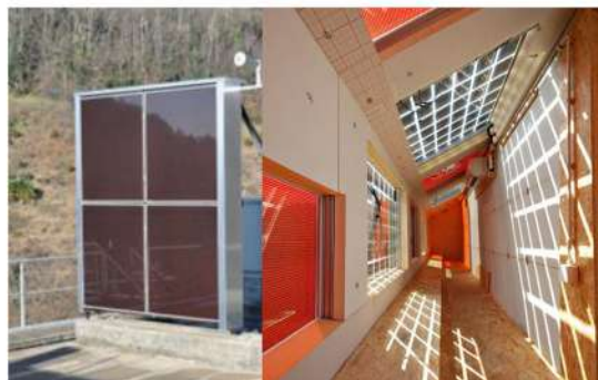
Figure 3: Examples of two different BIPV mock-ups from other authors for outdoor monitoring [6,7].
