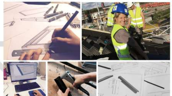
Figure 2: Developing process of Soltech ShingEI (solar tile) from sketches, making 3D drawings, creating prototypes, validation according to standards to negotiating suppliers, negotiating prices, making construction drawings, decide tolerances, set up production.
