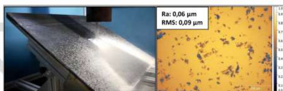
Figure 3: Sand blasting set-up; AFM measurement of sand blasted glass sample; AFM mobile device on the left side
