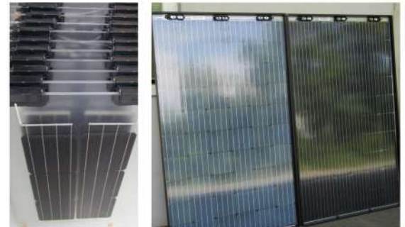
Figure 1: left: Specimens based on different material combinations; right: 60-cells standard PV modules with two different bifacial cell technologies and a glass-backsheet encapsulation
