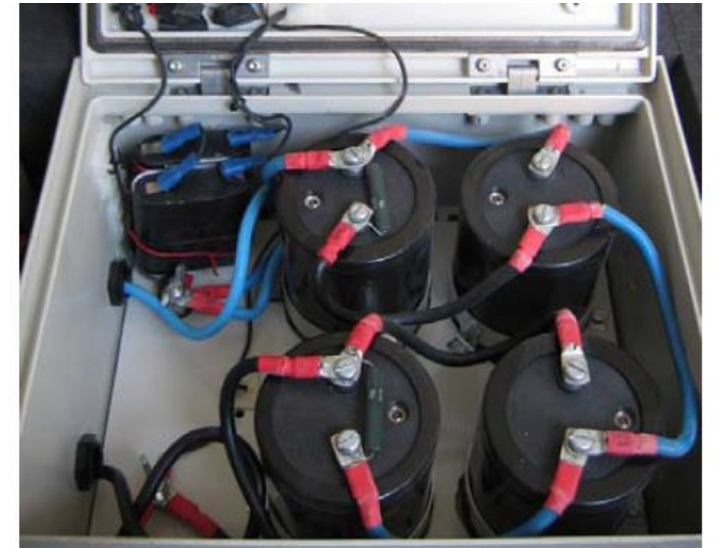
Capacitive load for I-V curves measurements (IES-UPM)
