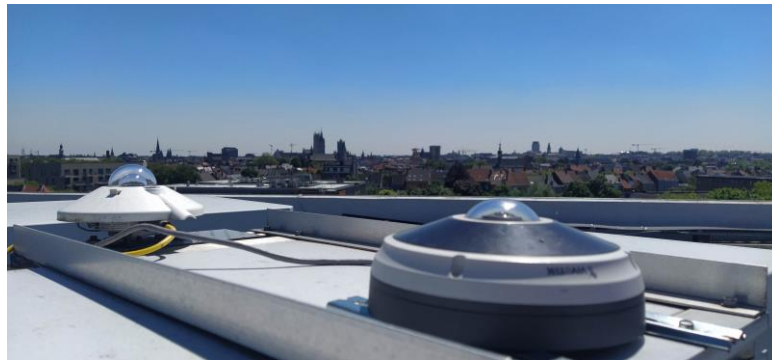
sky camera system operating in the visible spectral range with a fish-eye lens, KU Leuven
