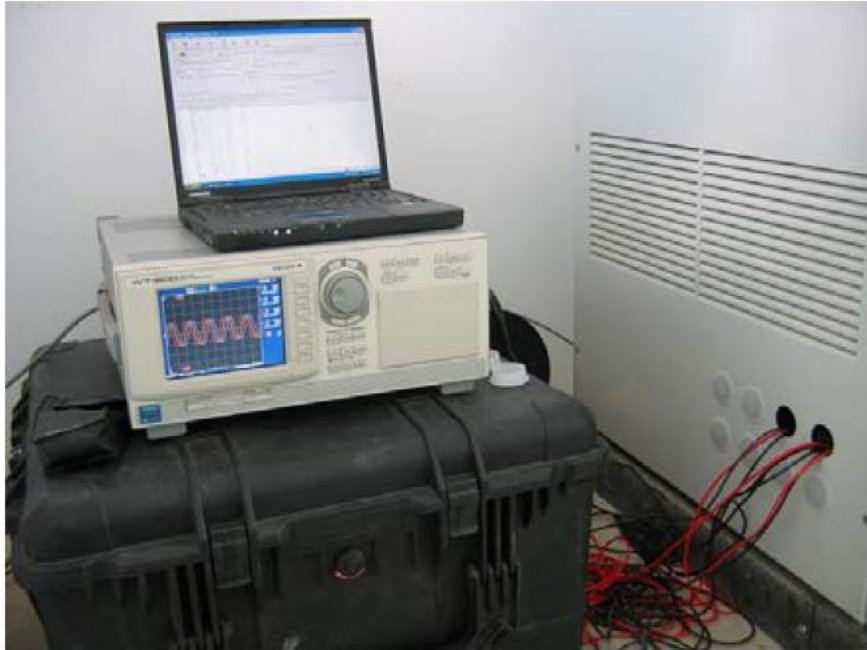
Wattmeter for power measurements (IES-UPM)
