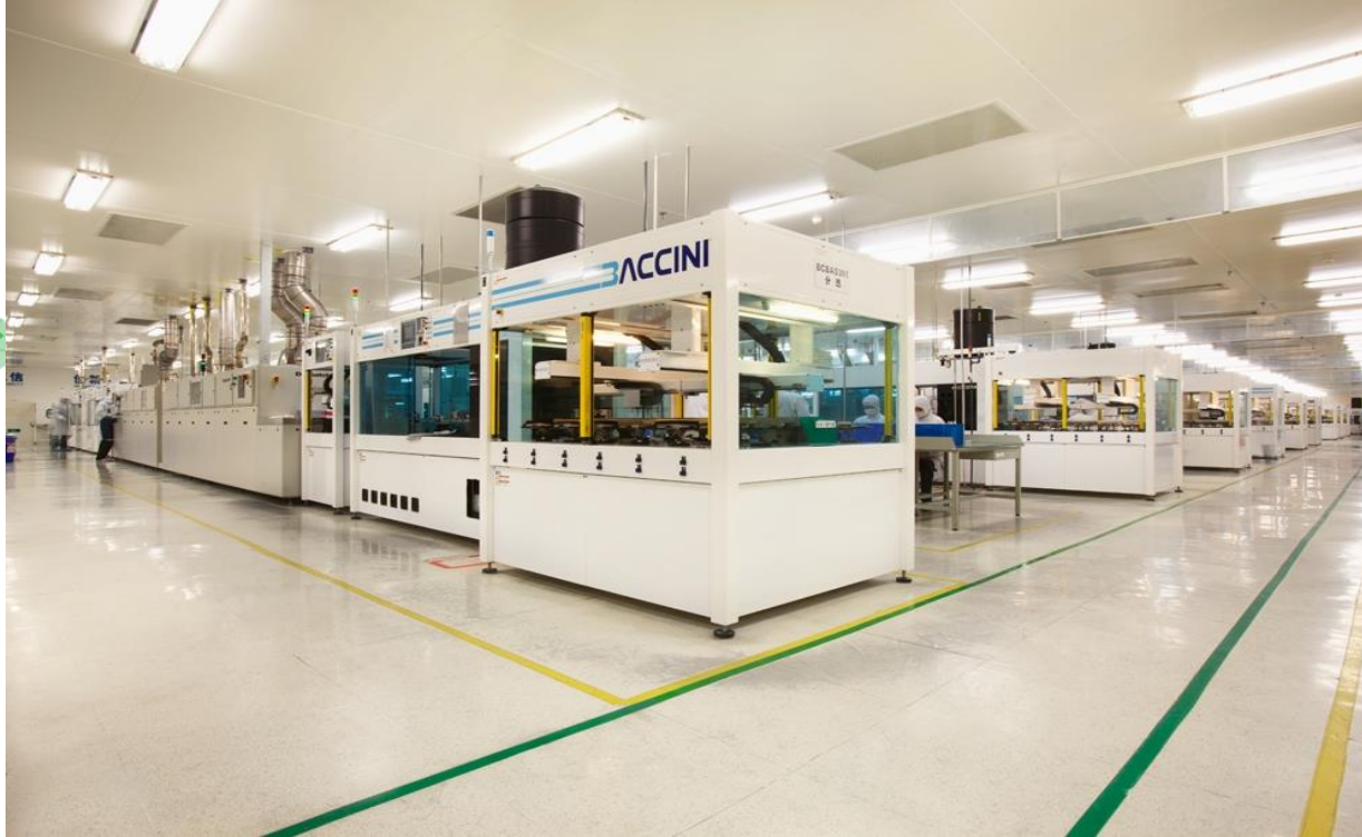
Figure 10.1.2 A screen-printed silicon solar cell manufacturing facility showing multiple production lines. Source: Courtesy of Trina Solar
