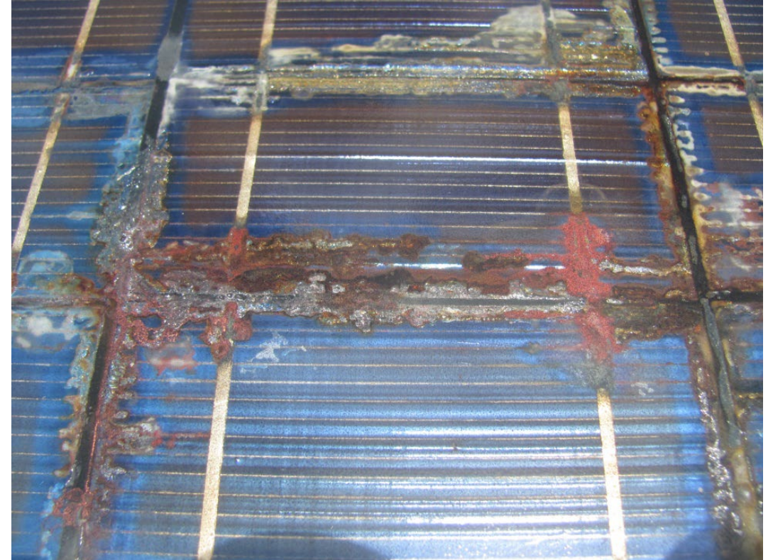
Silicon PV module after 22 years in Florida.
