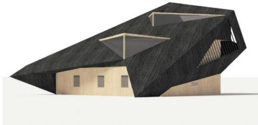
Up to the **80%** of the shell should be covered by PV panels in order to achieve the ZEB-OM ambition level
