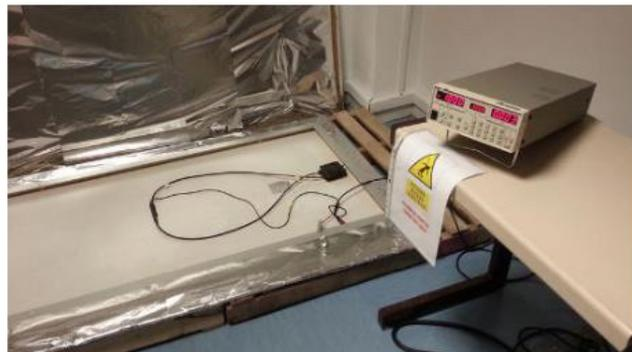
PID sensitivity test
