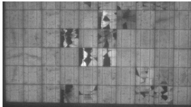
Electroluminescence of a module with fractured cells
