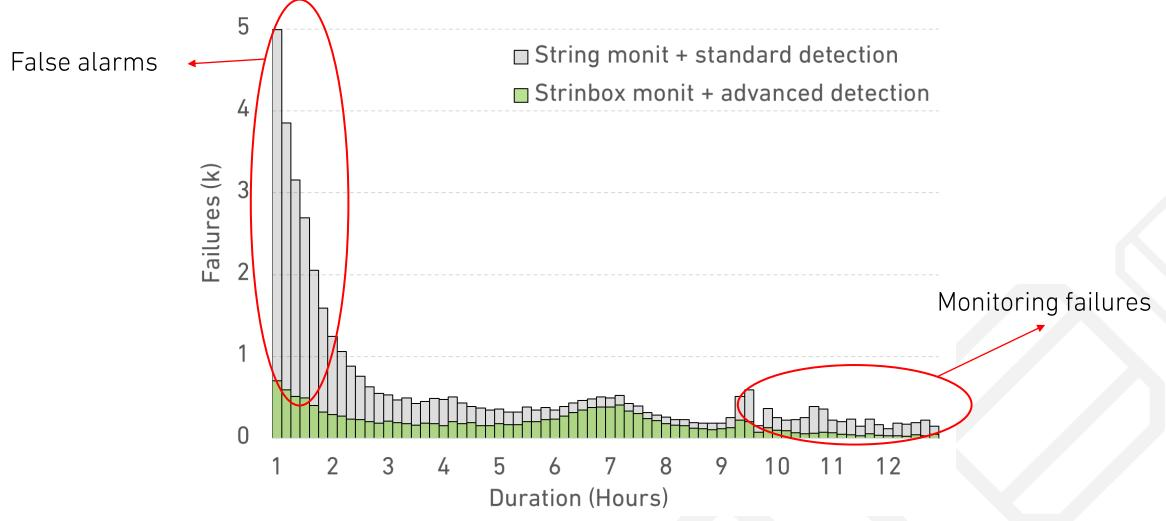
Detection +75% of the energy lost with only 5% of the sensors
