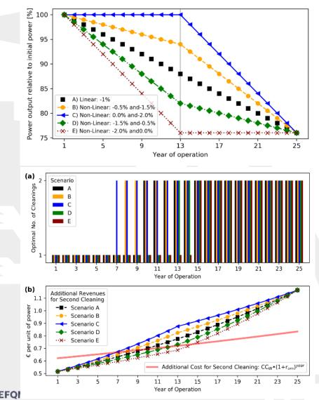
Five degradation scenarios were modelled, all resulting in 24% degradation loss after 25 years.
