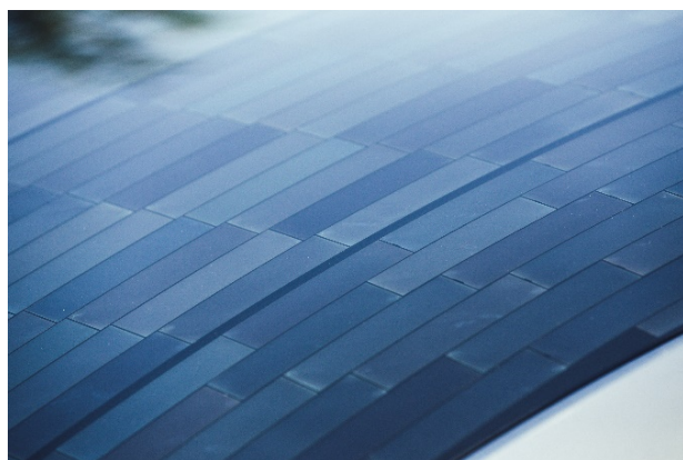
Integrated PV in car roof, courtesy of Lightyear.
