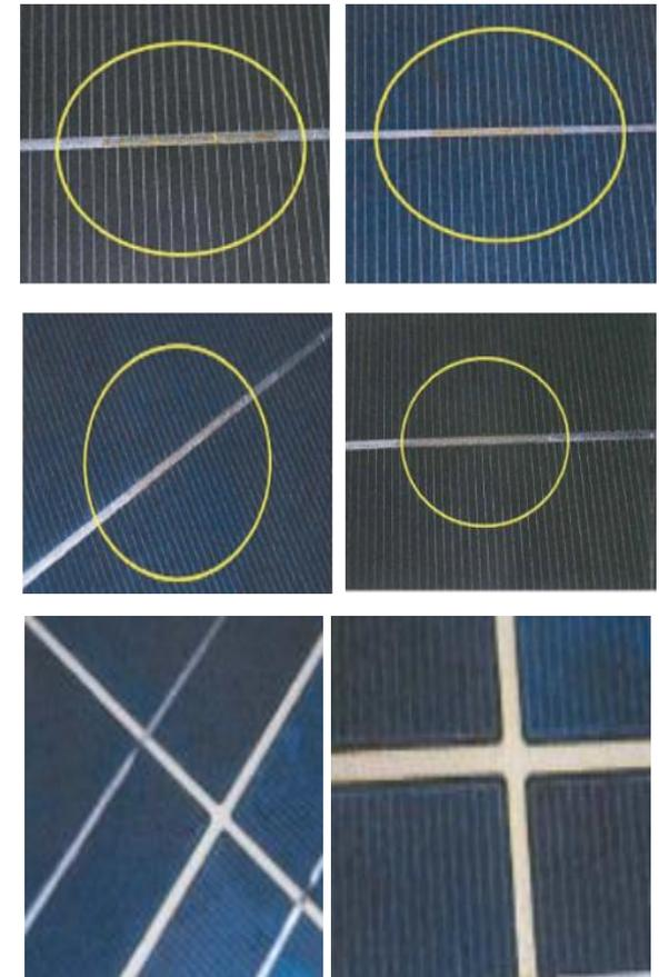
**Insufficient lamination parameters**
