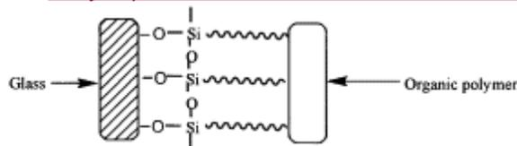
→ *Insufficient lamination may cause lack of adhesion*
