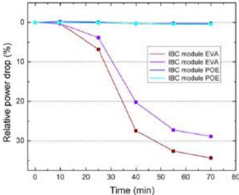
Figure 3: PID testing on Zebra mini-modules exhibiting POE and EVA as encapsulation material
