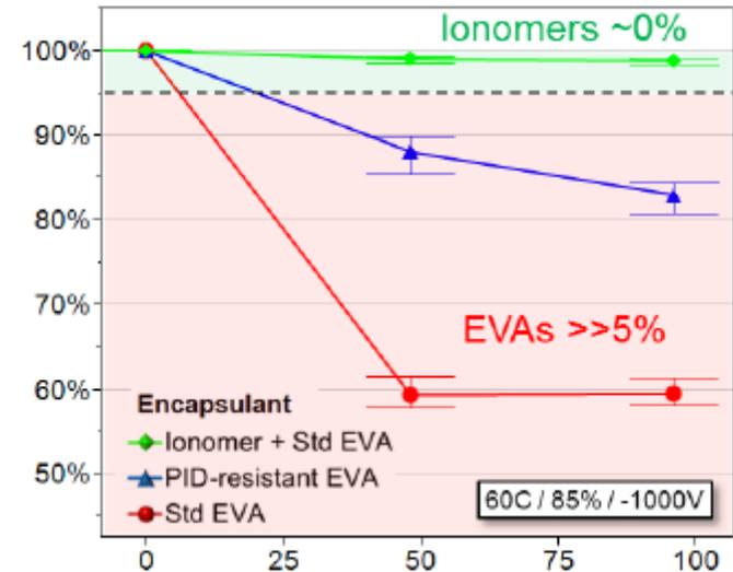
**Figure 6:** Comparison of relative output power for different encapsulants in 2nd set of nine full-size modules after PID exposure at 60 °C / 85 %RH / -1000 V of 96 hours. All modules were built at the Yingli production facility in Baoding, China.
