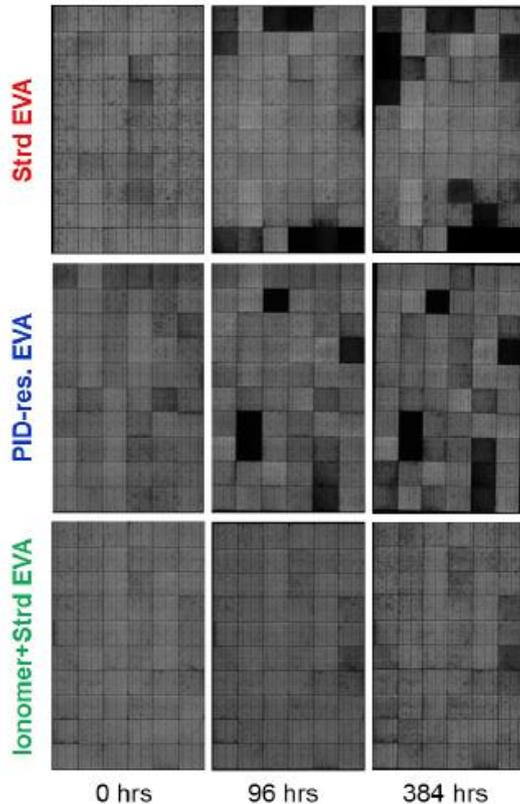
**Figure 3:** Electroluminescence images of full-size modules made with (i) Standard EVA (red circles), (ii) EVA designated as ‘PID-free’ (blue triangles), and (iii) an Ionomer film on top of a Standard EVA layer (green diamonds), after PID exposure at 85 °C / 85 % / -1000 V of varying duration.
