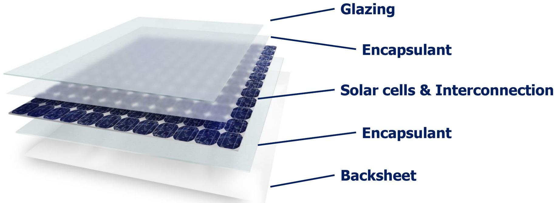
**Multi-material composite containing glass, polymers, semiconductors and metal**
